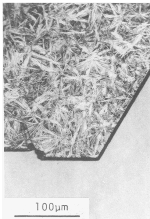
Figure 1 An optical micrograph of the deposit developed on a carbon surface of platy SiC single crystal.
